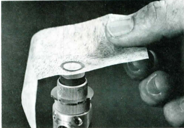
FIGURE 5.2: Cleaning the Mirror Surface
