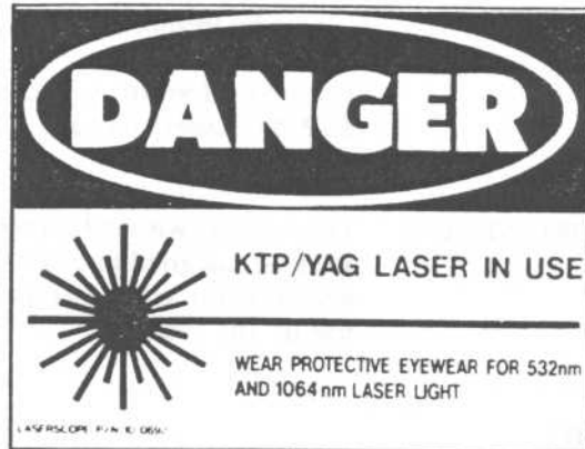
Figure 1-2 Warning Sign for KTP/532 laser with the Nd:YAG module operating at 532 nm and 1064 nm
