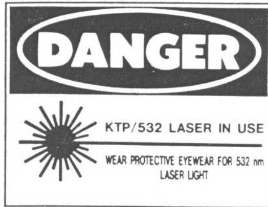
Figure 1-1 Warning Sign for KTP/532 laser operating at 532 nm only
