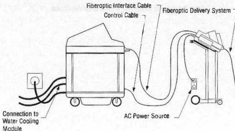
**Figure 2.3** Dye Module and Surgical Laser Connections.
