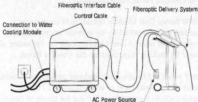
**Figure 3.1 Dye Module and Surgical Laser Connections**
