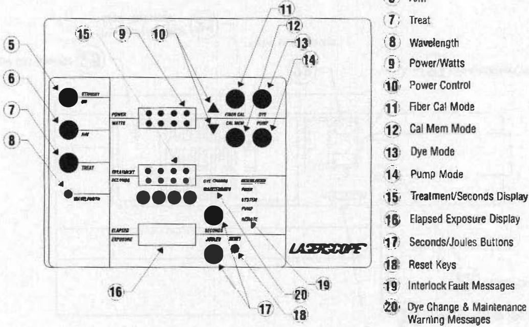
Figure 2. 5 Control Panel details and illuminating message screens.
