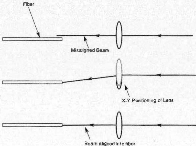
Figure 4.5: Fiber Alignment
