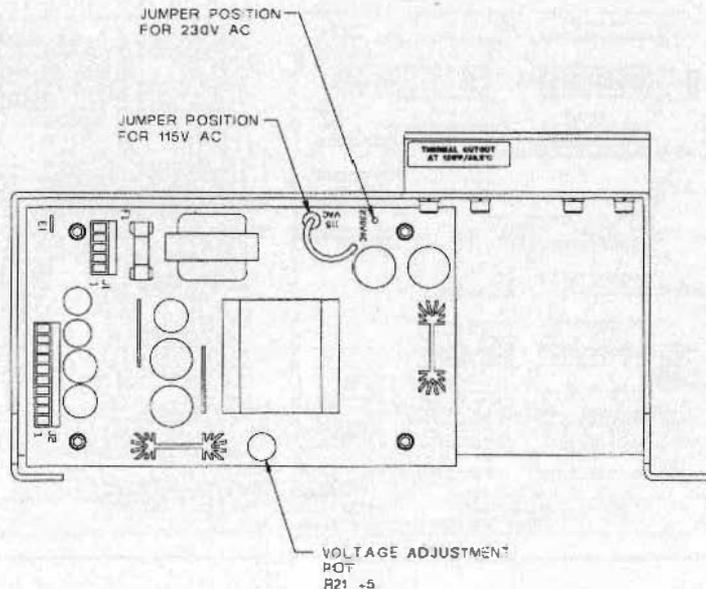
**Figure 5.3: Low Voltage Power Supply**
